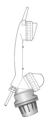
A manually operated electromagnetic call generator generates a warble current with a frequency of approximately 2000 Hz, which is transmitted directly to the transmitter capsule by a two-wire cable.
