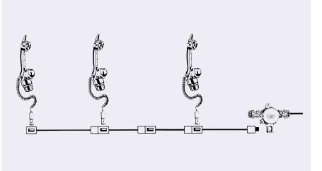
**2.** With movable telephone cable, with "prick pincers" – the quick connection from any part of the cable
