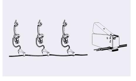
**3.** With firmly installed cable, for plug-connected hand telephones and/or permanently installed wall telephones
