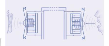
In principle only two capsules are needed to build a dynamic telephone system. An electric power supply is not necessary. The two capsules must be connected by any two-wire cable. Used as a microphone, the dynamic capsule generates a relatively high voltage from a low sound pressure. This voltage suffices to generate a sufficiently high sound pressure at the other capsule used as loudspeaker.
